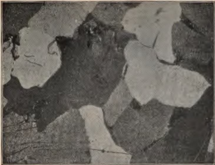
FIG. 1.—SOFT STEEL, 0.11% CARBON, ANNEALED. Magnified 130 diameters. Etched 1 minute in 0.1 nitric acid.
